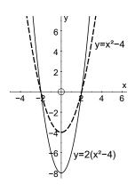
In general  $y = x^2$  or y = f(x) becomes  $y = ax^2$  or y = af(x) after a stretch in the y-direction of factor a.
