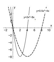
The new equation is formed by replacing x by  $\frac{x}{\frac{1}{2}} = 2x$  in the original equation.
